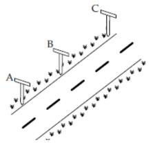
Determine whether or not the section of road ABC has been built in a straight line.
